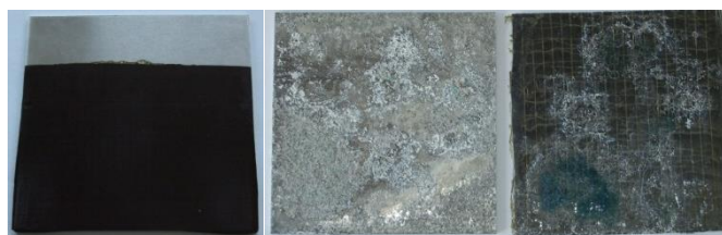
Figure 6: Alu-CFK sample coated (left) and not coated (right) after SST
